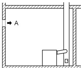
$$A = 150 \text{ см}^2 + 2 \frac{\text{см}^2}{\text{кВт}} \times (\Sigma \dot{Q}_n - 50 \text{ кВт})$$
